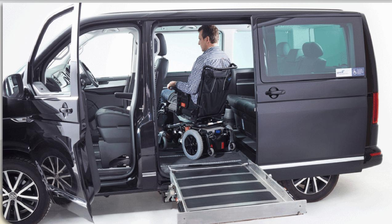
ACCÈS LATÉRAL DEPUIS UNE PLATE-FORME SOUS PLANCHER COMMANDÉE PAR UNE TÉLÉCOMMANDE
